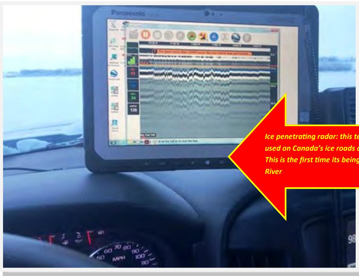
**Ice penetrating radar: this technology is already being used on Canada's ice roads and on Alaska's North Slope. This is the first time its being tested on the Kuskokwim River**
